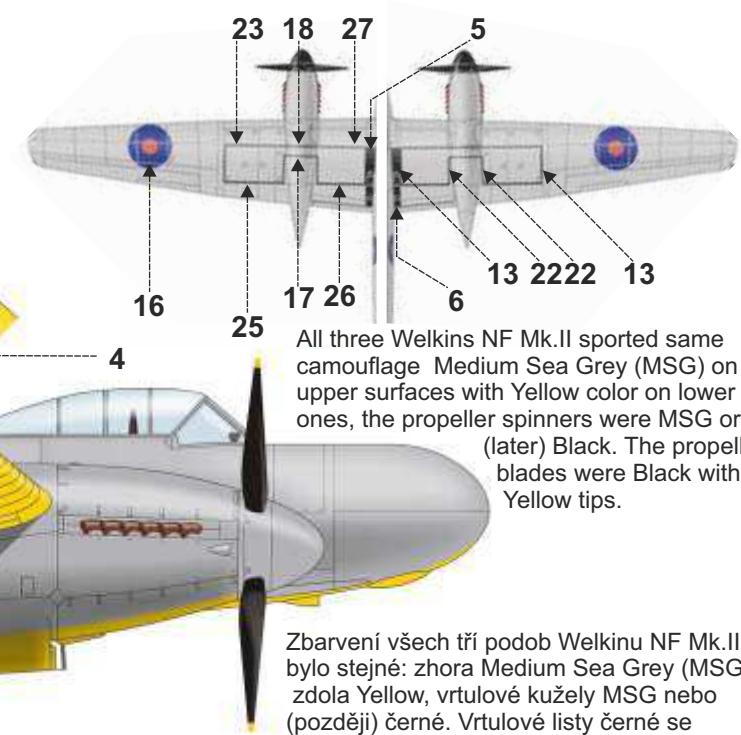
All three Welkins NF Mk.II sported same camouflage Medium Sea Grey (MSG) on upper surfaces with Yellow color on lower ones, the propeller spinners were MSG or (later) Black. The propeller blades were Black with Yellow tips.
