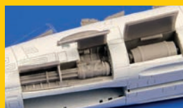
7453 F-14A Tomcat Port Side Cannon Installation
